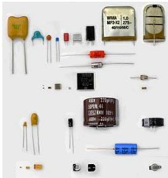
A **capacitor** (formerly known as a **condenser**, and prior to that known as a **permittor**) <sup>[1]</sup> is a passive two-terminal electrical component that stores electric energy in an electric field. The forms, styles, and materials of practical capacitors vary widely, but all contain at least two electrical conductors (called "plates") separated by an insulating layer (called the dielectric). Capacitors are widely used as parts of electrical circuits in many common electrical devices.
