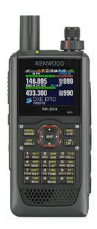
The FCC just released the test report for the new TH-D74 tribander, which I've attached. This new 144/220/440 HT will support D-Star, includes a built-in TNC and GPS and also has built-in Bluetooth and a MicroSD slot. The fact that the FCC has published the test results indicates that the radio should hit the market shortly. This looks like a very interesting radio that I can't wait to get my hands on.
