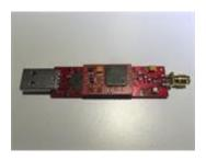
USB stick containing 70 cm data transceiver. This version contains an AMBE chip which allows the use of your PC's microphone and speaker to talk simultaneously to reflectors and through the DV4mini to other digital radios in range. DMR and DStar are supported with the
