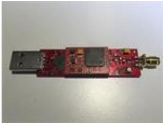
USB stick containing 70 cm data transceiver. This version contains an AMBE chip which allows the use of your PC's microphone and speaker to talk simultaneously to reflectors and through the DV4mini to other digital radios in range. DMR and DStar are supported with the AMBE chip. Fusion will be added later through a software upgrade. The other modes are supported like in the regular DV4mini using a handheld.
